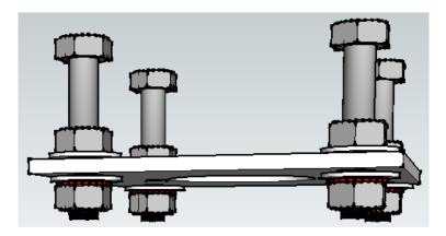
g) Mount the pump to the pump plate using [2] 7/16 bolts, nuts and washers:
