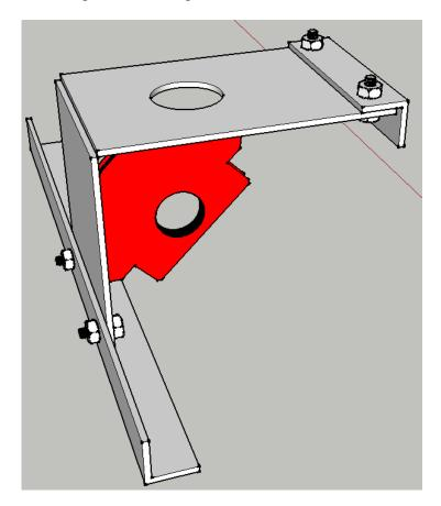
d) Mount the engine to the engine plate using [4] 5/16" x 2" bolts. The method for mounting may depend on your engine. See the following video for details:
