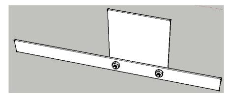
b) Bolt the  $\frac{1}{4}$ " x 8" x 12" plate to the 8" angle as shown using  $\frac{1}{2}$ " x 2" bolts:
