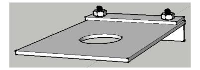
c) Align the plate edges and secure at 90 degree angle and weld. We use welding magnets to hold the plates at 90 degrees:
