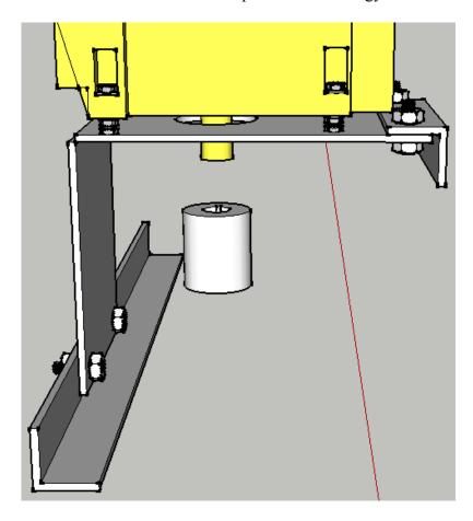
f) Assemble the 8" x 8" pump plate as shown with [4] 3/4" x 3.5" bolts and [8] 3/4" nuts, [8] washers and [4] lockwashers. Tighten the nuts to hold the plate firmly:
