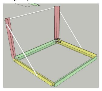
Note the corner holes that provide access for welding:
