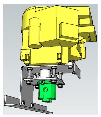
i) Lower the engine/pump assembly into the frame. Adjust it so the engine plate is parallel with the frame and weld the 8" angle iron to the reservoir and the 29" angle iron to the frame.
