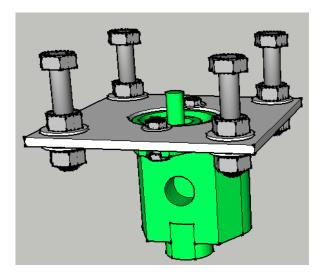
h) Make sure the key is in the pump shaft and slide the pump shaft into the bottom of the shaft coupling and tighten its allen screws. The bolt heads should just be touching the bottom of the engine plate. Tack and weld the bolt heads to the engine plate.
