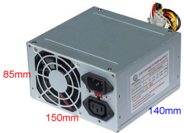
Standard ATX PS2 type. 85x150x140mm with an 8cm fan at front, On/Off switch, Volt switch, Monitor Outlet.
